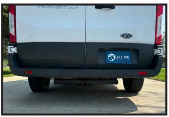
4. Ensure the hitch is centered and tighten all bolts.
