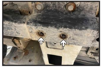
1. Clean area around existing holes using a wire brush. Then run a 12MM x 1.75 tap through the two (2) holes. Do this on both sides of the vehicle.
