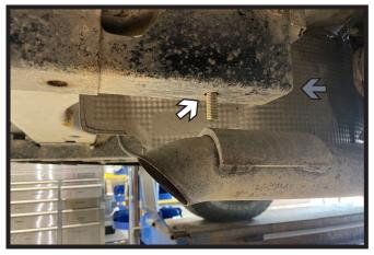
2. Place spacer plate onto 1/2" carriage bolt. Slide bolt and plate through forward access hole (gray) in the frame. Place bolt (white) in forward hole so that plate is flush with the frame and bolt hangs vertically. Do this on both sides of the vehicle.
