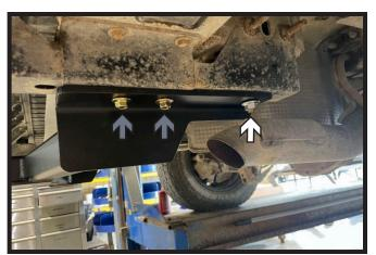
Raise hitch into place. Install whiz nut (white) onto 1/2" carriage bolt, leave loose. Then install the two (2) 12M-1.75 bolts (gray) into the existing holes, leave loose. Do this on both sides of the vehicle. Note: If needed, lower the exhaust on each side to allow more room to install whiz nuts.
